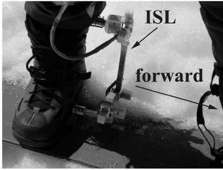
**Fig. 7** The ISL mounted to the right snowboard boot of the subject performing a heel-side turn with a regular stance. Also visible are the ISL sole mount and cuff mount, along with the ISL data cable which travels up the right leg and into a backpack.
