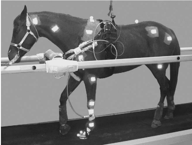
Fig. 3. Photograph of Thoroughbred mare with the dynamometric horseshoe trotting on the treadmill. The reflective markers were not used in the present study.
