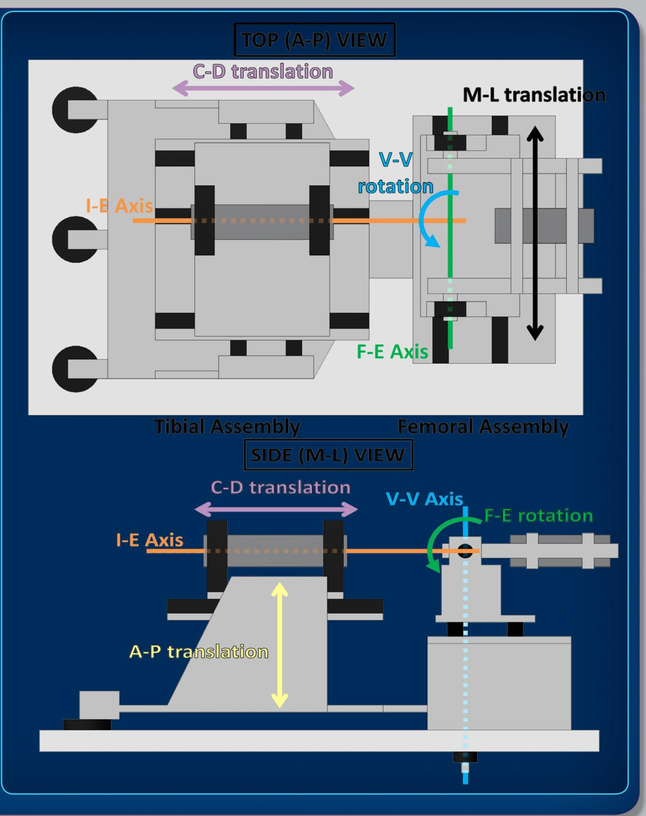
The applied loads used to define the limits of passive motion were  $\pm$  3 N-m for I-E rotation<sup>2</sup>,  $\pm$  5 N-m for V-V rotation<sup>3</sup>,  $\pm$  45 N for A-P translation<sup>4</sup>, and  $\pm$  100 N for C-D translation<sup>5</sup>. Throughout testing, a 45 N compressive
