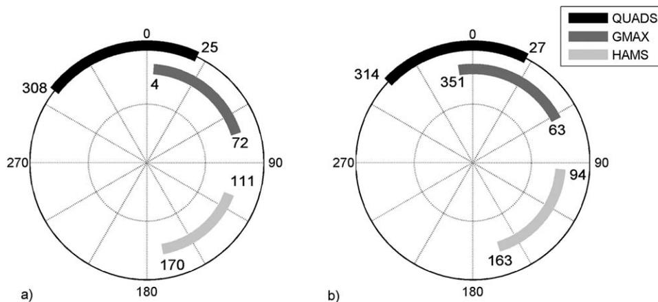
**FIGURE 1.** Plot of muscle electrical stimulation on and off timing as a function of crank angle for the: **(a)** commercially available electrical stimulation ergometer (StimErg); and **(b)** the minimized stress-time integral for the quadriceps (QUADS), gluteus (GMAX), and hamstring (HAMS) (Stim3) muscle groups. Top-dead-center indicates 0° and the beginning of the crank cycle. The on and off timing angles are listed at the beginning and end of the stimulation for each muscle group.
