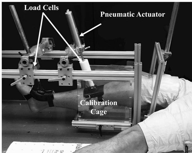
**Fig. 2** Photograph showing the limb in the loading apparatus. The knee was centred in the calibration cage and was flexed 25°. The ankle and thigh were secured in supports. The pneumatic actuator was oriented perpendicular to the shank and parallel to the knee joint at a distance of 12.5 cm distal to the joint line. The pneumatic actuator applied anterior and posterior forces to the tibia. Load cells measured the applied force and the reaction force at the ankle joint [39]
